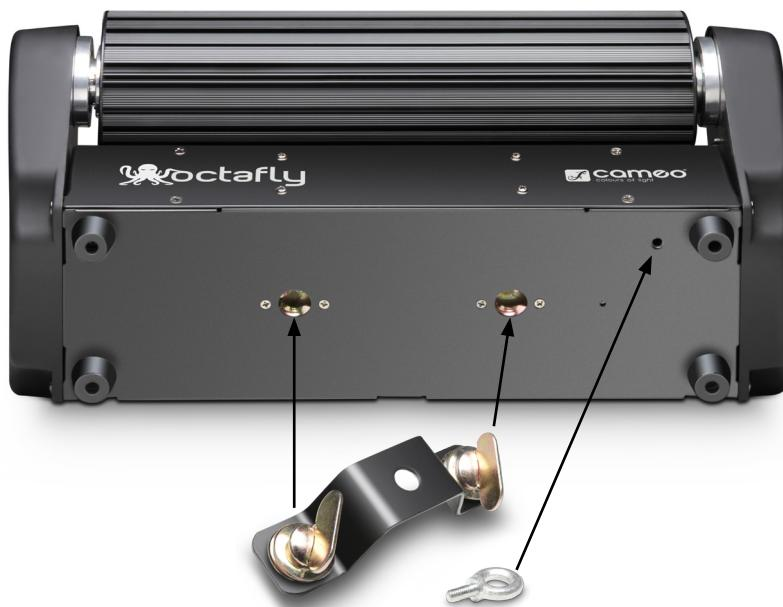
**EN** Thanks to the integrated rubber feet, the spotlight can be placed in a suitable location on the stage floor etc. Mounting on a truss is performed with the help of the supplied omega mounting bracket; secure the device with a suitable safety rope to the safety screw eye. NOTE: Overhead installation should only be carried out by trained personnel.
