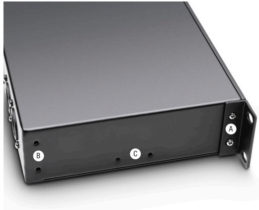
**EN** For an individual rack mounting, the rack-mounting brackets can be mounted both to the front (A), as well as to the rear (B) of the device. Wall mounting, or under table mounting is possible using the thread in the middle of the housing side (C). Only use the original screws to fasten the rack mount bracket.
