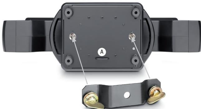
**EN** Thanks to the integrated rubber feet, the spotlight can be placed in a suitable location on the stage floor etc. Mounting on a truss is performed with the help of the supplied omega mounting bracket and a suitable truss clamp (not included). Make sure that the connection to the device is solid and secure the device with a suitable safety rope to the safety screw eye (A). Important Notice: Overhead installation should only be carried out by trained personnel.
