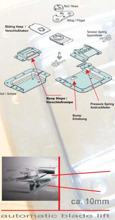
This new patent pending Butterfly is the first of a new generation of flight case latches, featuring a fully new "no push, no protrusion" system **A** which automatically guides the blade hook into the keep slot.
