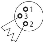
Termination reduces signal transmission problems and interference. It is always advisable to connect a DMX terminator, (resistance 120 Ohm 1/4 W) between pin 2 (DMX-) and pin 3 (DMX+) of the last fixture.
