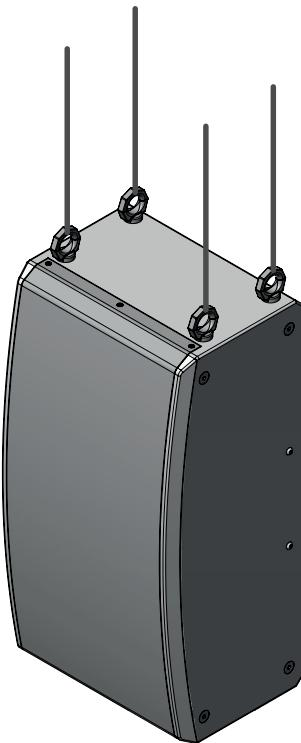
**EN** Attach suitable steel ropes, or steel chains to the 4 eyelets (suitable ring screws, eye nuts etc.) to the chosen location on the ceiling in such way that they are parallel to each other (same hole spacing as the ring screws on the subwoofer). Make sure that the steel ropes, or steel chains have the same length and secure them with the appropriate connectors onto the ring screws of the subwoofer.
