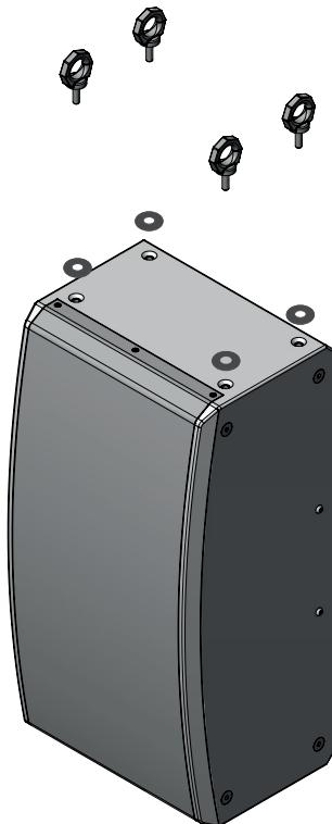
**EN** Screw one ring screw into each of the 4 M8 threaded sleeves in the corners on the chosen mounting side (short or long side of housing). For this purpose, use M8 ring screws with at least 20 mm of thread length and use a 24 mm washer to enlarge the surface of the ring screw head (ring screws and washers not included). Ensure a tight fit.
