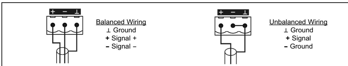
Important!: If a connection is done with a un-balanced line and pin - on the Euro style is not connected to ground, a 6 dB loss occurs in the line and only a quarter of the amplifier power is produced.
