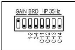
**Sub-sonic Filter Enabled:** the amplifier works with Channel 1 high pass subsonic filter (35Hz), 32dB Gain and no Bridge mode.
