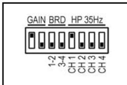
**Bridge Mode:** the amplifier works without high pass subsonic filter, 32dB Gain and Channel 1/Channel 2 Bridge mode.
