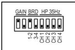
**Gain Selection:** the amplifier can work at 26dB, 32dB or 38dB Gain.
