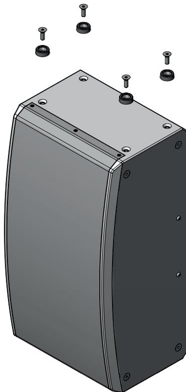
**EN** Unscrew the 4 screws from the M8 threaded sleeves in the corners (short or long side of housing) on the chosen installation side; screw the included rubber feet to the corners and place the subwoofer at a suitable location on a level surface.
