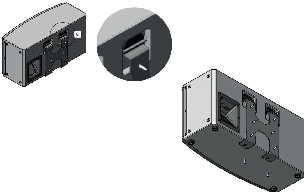
**EN** 3. Using the supplied M6 retaining screws, screw on the mounting bracket and subwoofer; do not use the previously removed countersunk head screws for this purpose. Ensure a tight fit.
