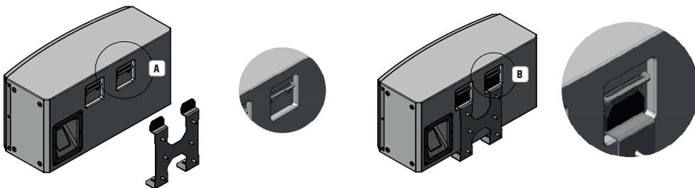
**EN** 2. Remove the two countersunk head screws (M6) at the bottom of the subwoofer and connect the speaker cable BEFORE mounting the subwoofer to the corresponding connection. Now guide the subwoofer as shown onto the mounting bracket and slide it in the direction of the mounting angle. Make sure that the retaining tabs on the mounting bracket are correctly positioned in the support lugs of the subwoofer (see Figures A, B and C).
