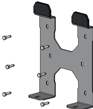
**EN** 1. Screw the mounting bracket onto a solid wall or ceiling at the chosen location (for wall mounting with the support lugs upward). Please make sure to use appropriate screws and ensure a firm hold.
