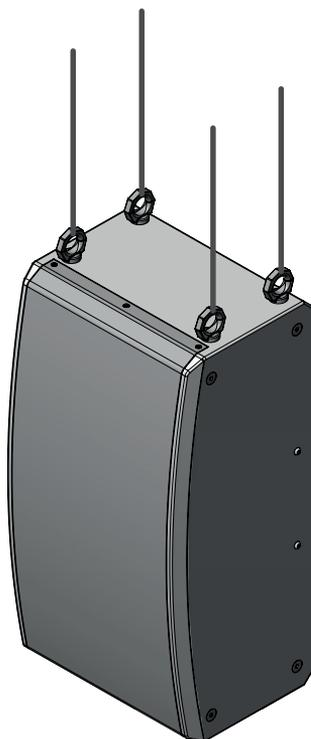
**EN** Attach suitable steel ropes, or steel chains to the 4 eyelets (suitable ring screws, eye nuts etc.) to the chosen location on the ceiling in such way that they are parallel to each other (same hole spacing as the ring screws on the subwoofer). Make sure that the steel ropes, or steel chains have the same length and secure them with the appropriate connectors onto the ring screws of the subwoofer.
