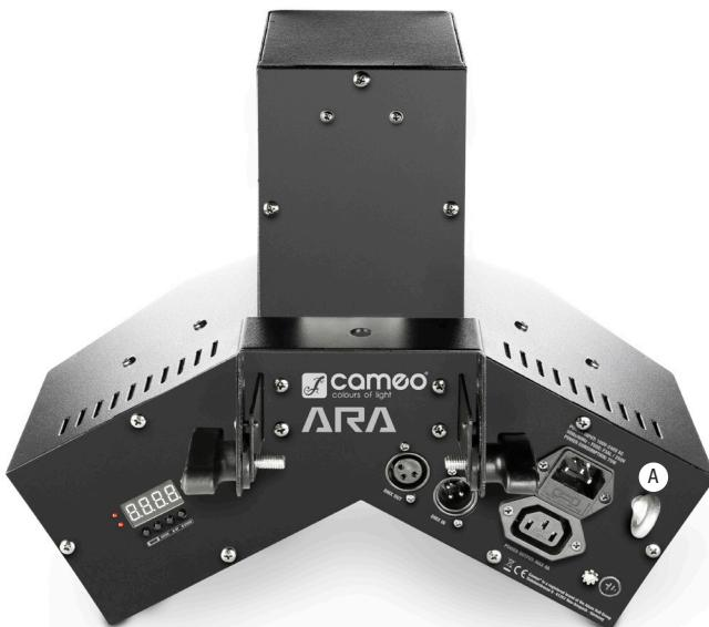
**EN** Mounting on a truss is performed using a suitable truss clamp (not included) and the integrated mounting bracket; secure the device with a suitable safety rope to the safety eyelet A. Overhead installation should only be carried out by trained personnel.
