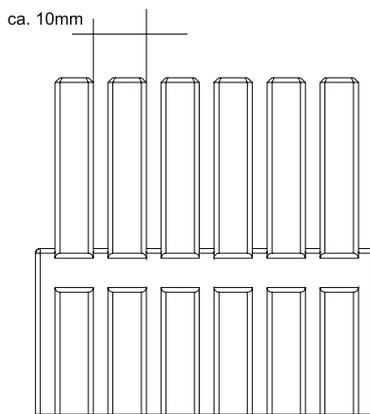
Partitioning system for all Drawers. The interlocking partitioning strips can be individually used to divide the drawer compartment into smaller sections as required by shortening the strips length in 12 mm increment - using our „score-and-snap“ feature.
