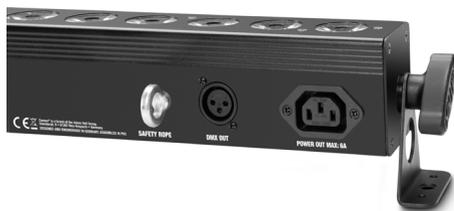
The Cameo Tri Bars can be mounted using the mounting bracket on the left and right-hand side of the housing, either in a convenient location on the floor or similar, or on a truss system (truss clamp not included). Please use the safety eyelets on the housing to secure the spotlight against falling down. NOTE: Overhead installation should only be carried out by trained personnel.
