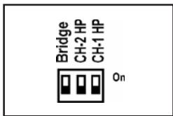
**Sub-sonic Filter Enabled:** the amplifier works with Channel 1 high pass subsonic filter (35Hz), and no Bridge mode.
