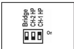
**Bridge Mode:** the amplifier works without high pass subsonic filter, and Channel 1/Channel 2 Bridge mode.
